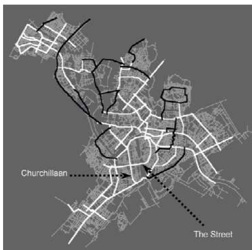
Figure 4. The representation of complete supergrid network (white lines are the supergrid that emerges out of the fabric, the black lines are the engineered supergrid network)
